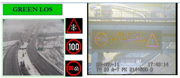
Figure 1.- Image of the road network with green level of service. On the right, the signals used in VMS.
